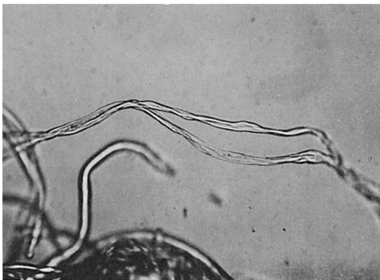
Fig. 7. Optical micrographs of fibers after immersion in mineral oil (a), water (b), and 0.5M cuene (c). Fibers from a DEAE-cotton of 4.47% N that was reacted with diiodopentane to form the diquaternaryammonium cellulose iodide and then converted to the thiocyanate form in nonaqueous media.
